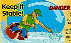
Leaning shoulders outside the edge of the boat can lead to a capsize. Keep your weight low and balanced over the centerline of the boat.
